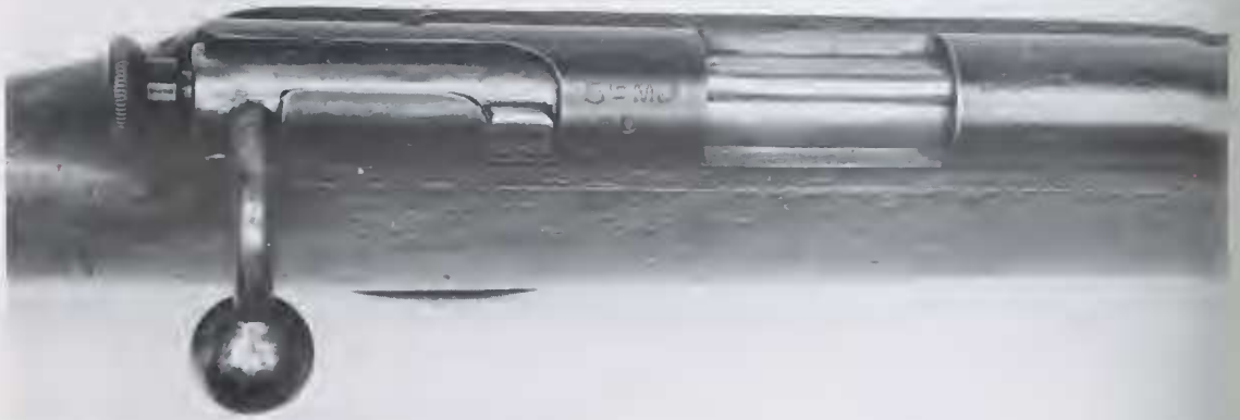
Figure 32 The breech of the rifle illustrated in Figure 31, showing the repeated stand number and issue marks for Western Australia. (Photo D. Elford).
